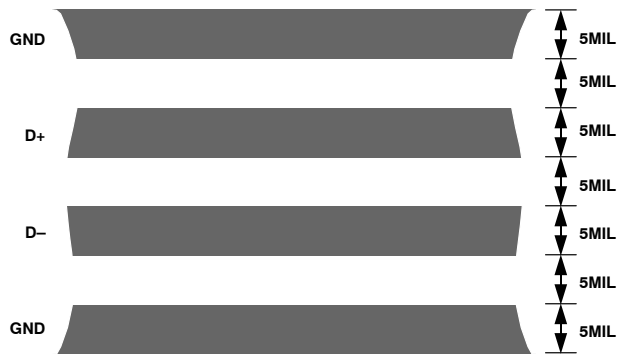
Figure 16. Typical Arrangement of Signal Tracks
